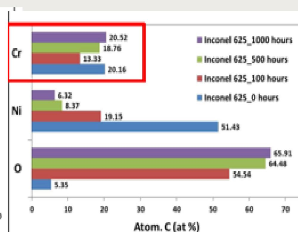
**Test Conditions:** 850 °C; 6.0 L/min Airflow; 3 vol% H<sub>2</sub>O.
